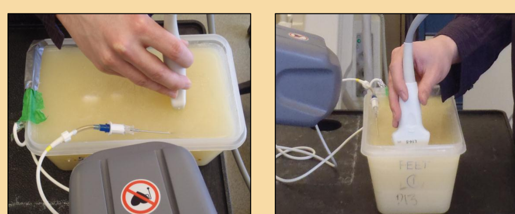
Figure 4: US data being collected on a spine phantom
