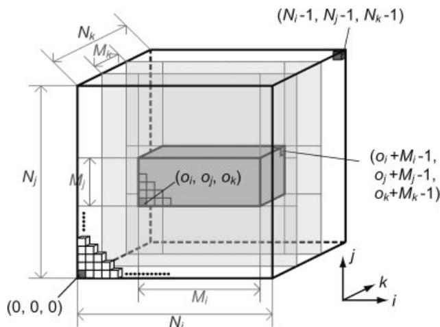
**Figure 1.** Parameters to support partial 3D volume update. The outer cube denotes the entire range of the 3D image, and the inner cube denotes the partial 3D image that is contained in the message as a byte array
