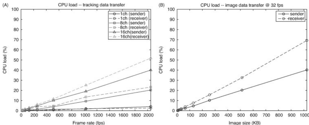
**Figure 4. (A) CPU loads during tracking data transfer are compared among 1-, 8- and 16-channel tracking. Comparison is also made between sender and receiver. (B) CPU loads during the image data transfer are compared between sender and receiver**
