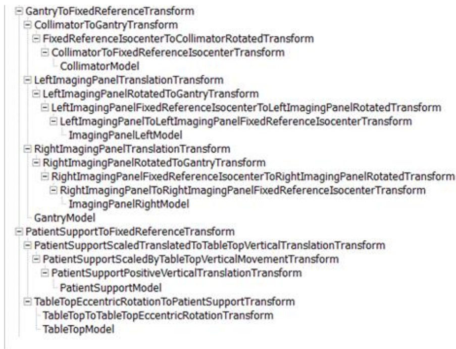
Figure 3. The transform hierarchy for EBRT machines defined in the IEC standard implementation in 3D Slicer using the matrices representing rigid transformations.
