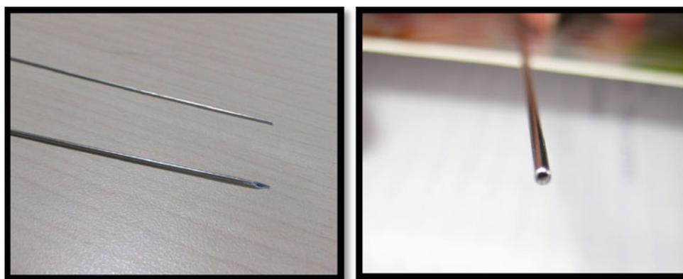
**Fig. 4** *Left* Catheter on *bottom* and needle analogue on *top*. *Right* Close-up image of catheter analogue
