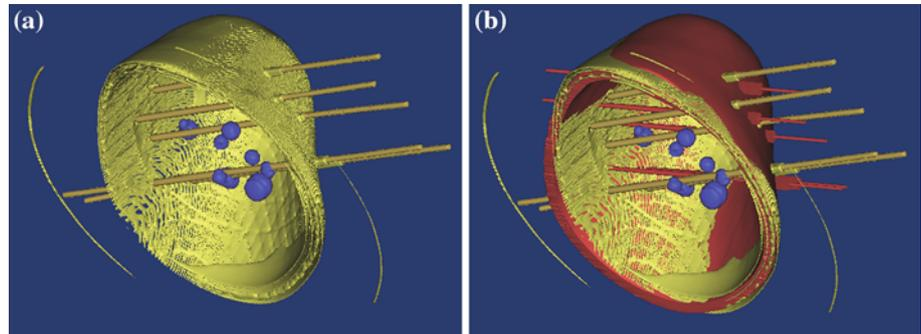
**Fig. 8** Screen shots from *Magic*. Model of pre-operative template plan ready for printing. *Left a* shows the lengthened guide tracks implemented on template. *Right b* displays guide tracks as well as three fiducial guides that appear as spherical bumps along the bottom edge of the template
