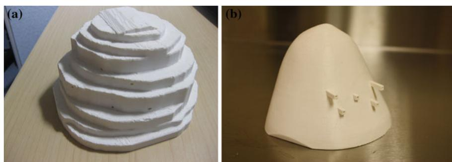
**Fig. 6** Templates created using 3D rapid prototype printer *Left a* first template designed and printed for catheter guidance. *Right b* template printed during second round of experimentation with improvements to template made
