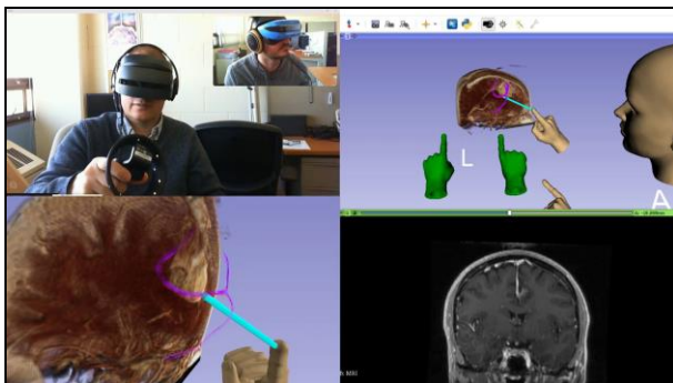
Fig. 3 Remote VR collaboration for brain surgery planning using real-time tractography. Top left: Participants local (blue headset) and remote (black headset). Bottom left: VR mirror image (local). Top right: 3D view of the SlicerVR instance (local). Bottom right: coronal slice in the position of the tractography seed (local). Introduction video: https://youtu.be/rG9ST6xv6vg
