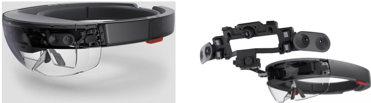
Fig 1. Microsoft HoloLens headset (left). The four environment understanding cameras and one depth camera built into the HoloLens (right) 10 .
