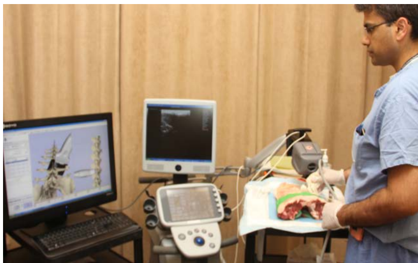
Figure 6. Tracked ultrasound for biopsy navigation with 3D Slicer. US imaging and tracking data are acquired by PLUS and streamed to 3D Slicer for live display.
