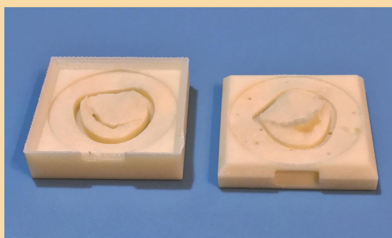
Fig 6. 3D-printed bottom mold and top mold for a mitral valve (step 3)
