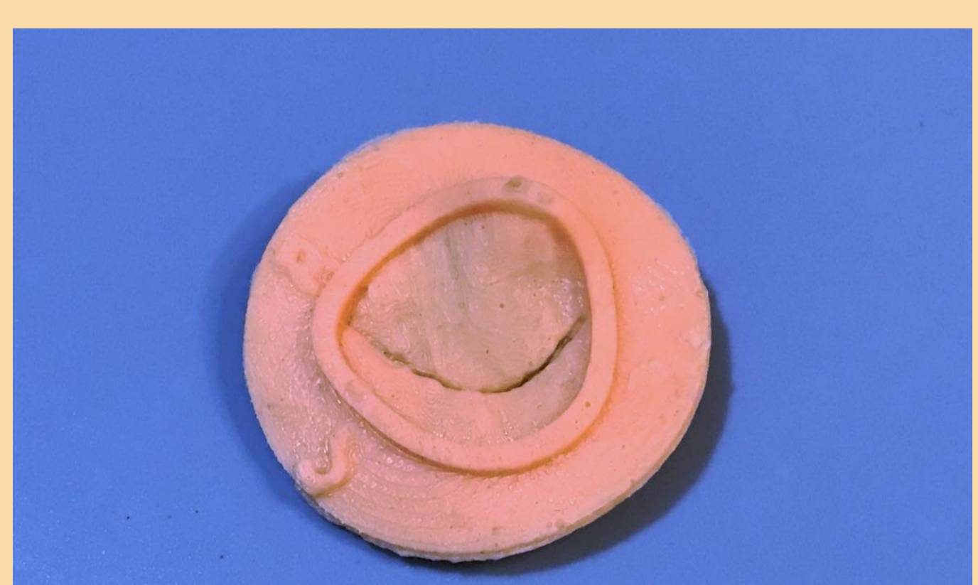
Fig 7. Silicone mitral valve created from mold (step 4)
