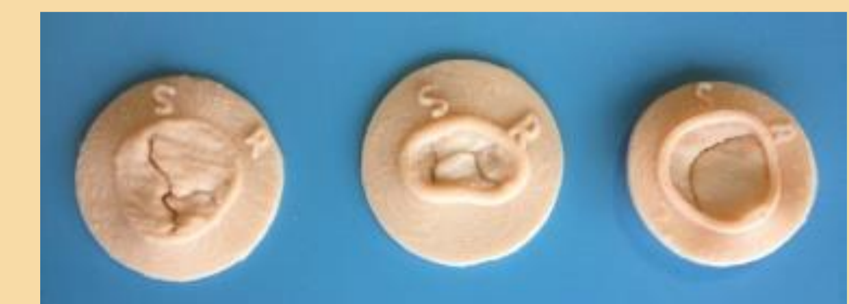
Fig 9. Silicone valve models left to right: tricuspid, complete atrioventricular canal defect, mitral
