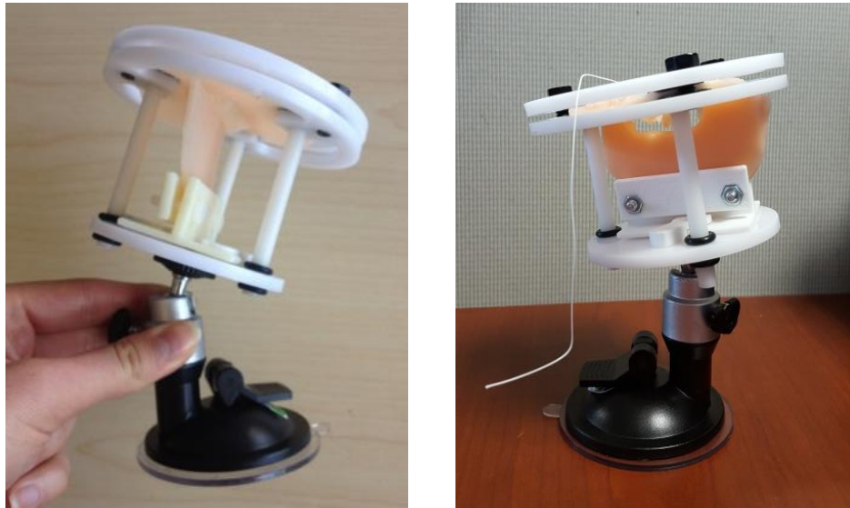
Figure 8. Setup for CAVC repair simulation: a CAVC valve model is secured at the top of the valve holder. A silicone ventricular septal model is secured below the valve with a separate 3D-printed holder.
