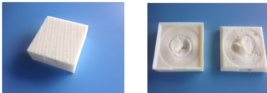
Figure 6. 3D-printed mold for a tricuspid valve (case B): assembled (left), and disassembled (right).
