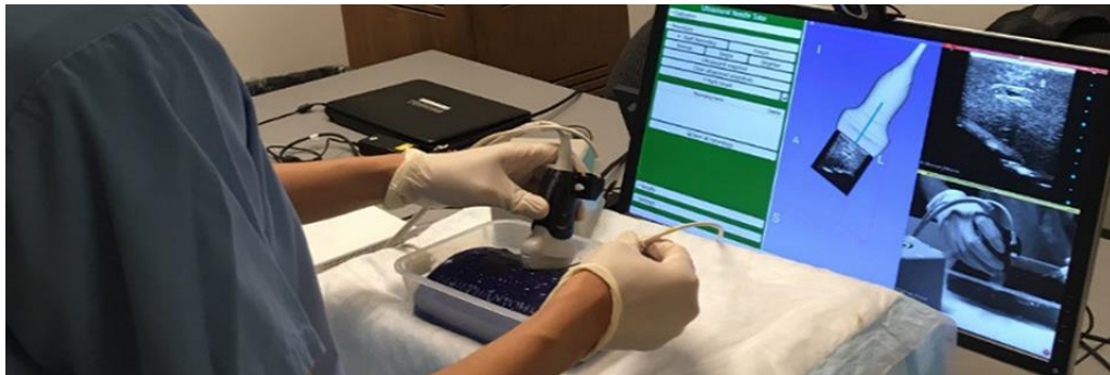
Figure 1. Trainee practicing out-of-plane needle insertion under ultrasound-guidance with augmented reality 3D display.
