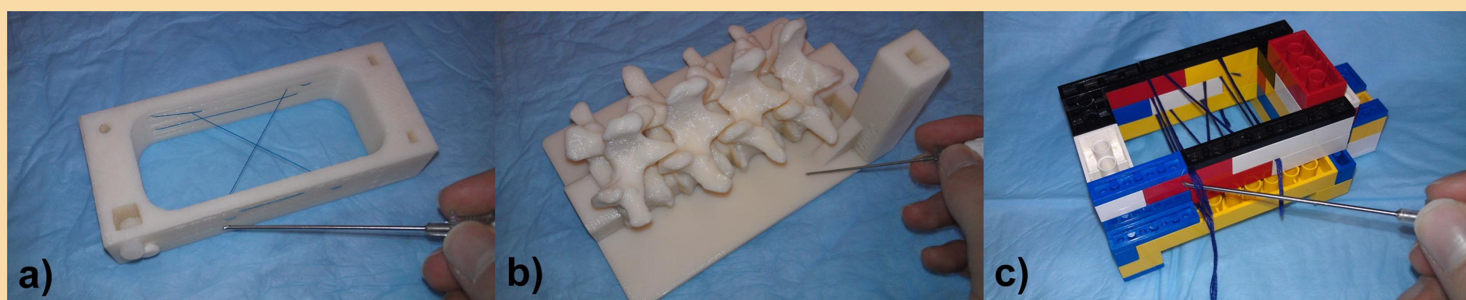
Figure 1. Photograph of user collecting points on the a) fCal phantom [1], b) lumbar spine phantom [3], and c) LEGO® brick phantom [4].
