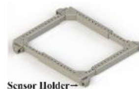
Figure 1. Mechanical design of the frame to hold Ascension EM sensors.
