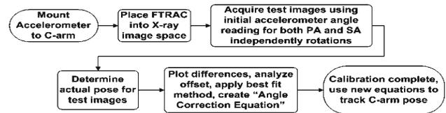
Fig. 3 The steps for C-arm pose tracking with accelerometer. PA primary angle, SA secondary angle
