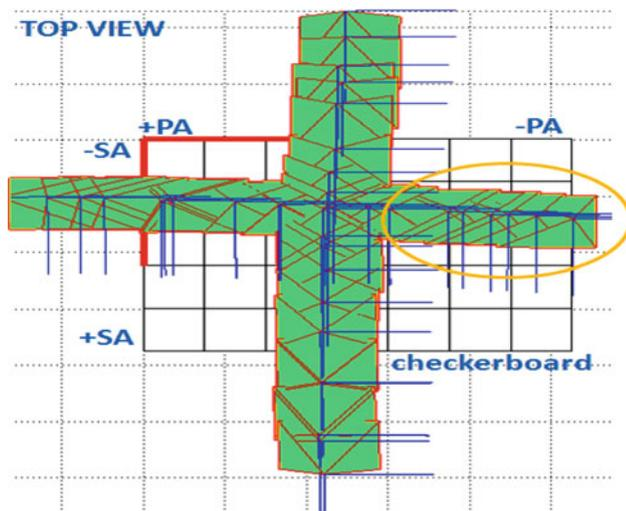
**Fig. 7** The distribution of the pose of calibration images for the webcam C-arm metal analogue. The circled highlighted area shows a slanting path during negative PA rotation, which creates an unaccounted for offset when rotating diagonally
