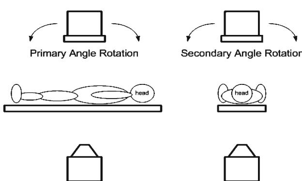
**Fig. 1** C-arm rotational axes relative to the placement of patient
