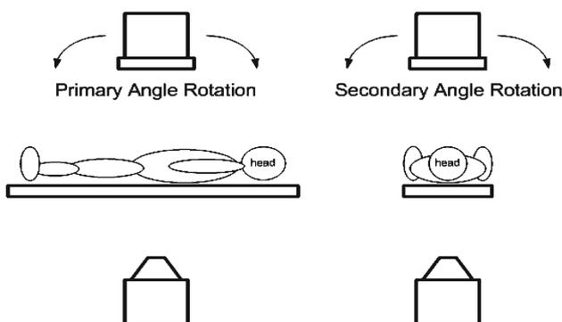
**Fig. 1** C-arm rotational axes relative to the placement of patient
