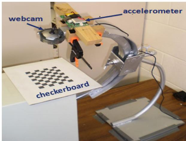
**Fig. 4** Experimental setup for the C-arm analogue with checkerboard plate for calibration and ground-truth for pose tracking
