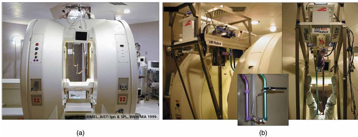
Figure 3. (a) GE Signa SP open-MRI scanner, with (b) integrated 5-DOF MR-compatible robot. The robot end-effector is equipped with an optical tracking marker (inset).
