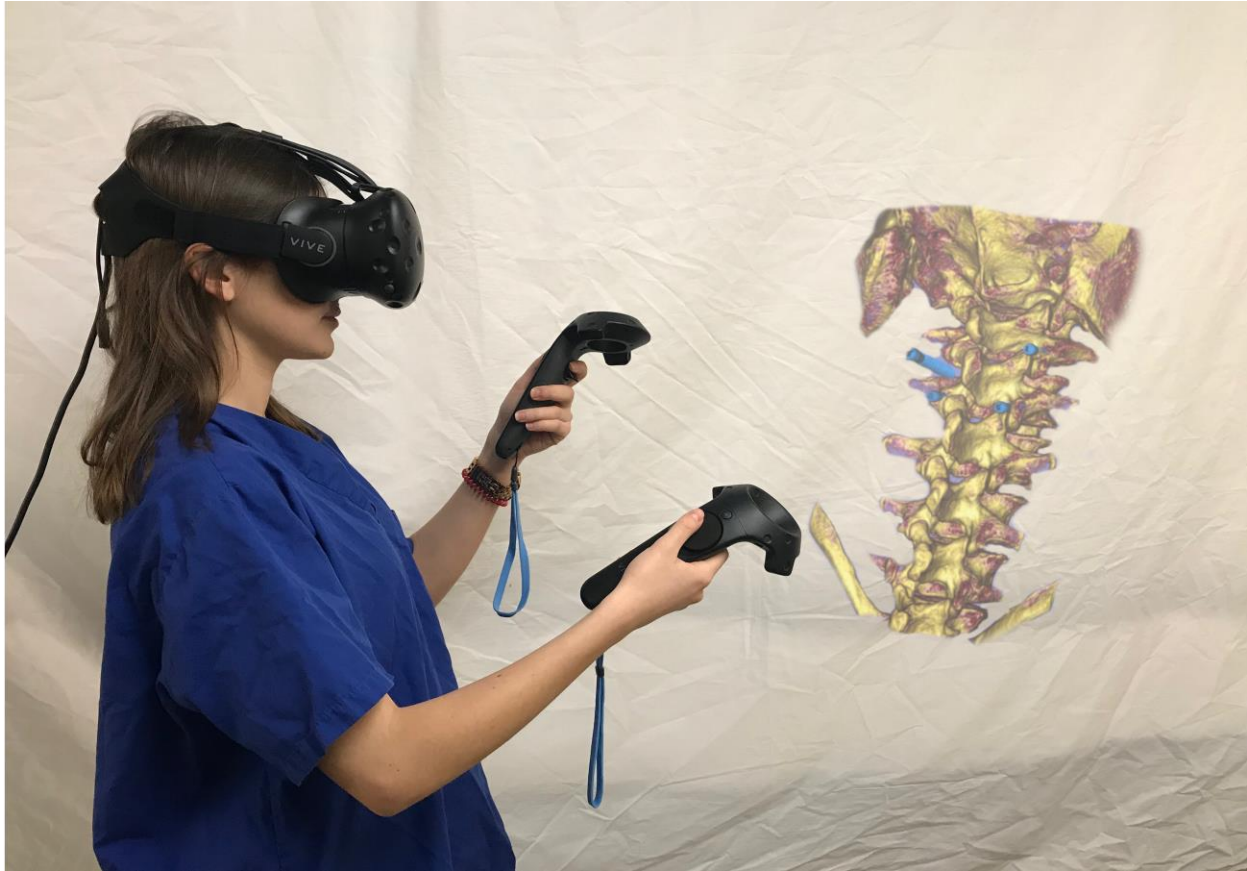
Figure 3: The HTC Vive Head-Mounted-Display and controllers being used to navigate a virtual scene that consists of a spine volume rendering used for pedicle screw insertion.
