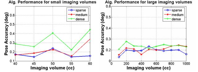
Figure 3. Relative pose error as a function of the imaging volume for small volumes(left) and large volumes (right)
