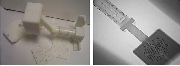
Figure 4. An image of the point phantom attached to the FTRAC fiducial (left). A typical X-ray image of the combination (right)
