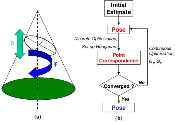
Figure 1. Graphical representation of the angles phi and theta, used to slice the cone and obtain an ellipse(left). Algorithmic flowchart showing pose estimation with point correspondences (right)
