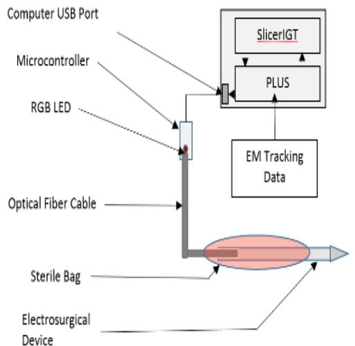
Figure 2: Schematic of Visual Feedback System
