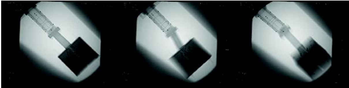
Figure 1. Fiducial device containing wire ellipses, and seed cloud phantom to be used in assessing algorithm. Within the phantom cloud block are precisely positioned sample seeds.
