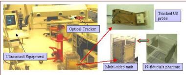
Figure 3: Calibration setup shows the multi-sided tank with the N-fiducials
