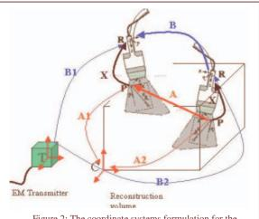
Figure 2: The coordinate systems formulation for the proposed AX =XB method.
