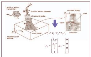
Figure 1: The chain of transformations is from pixel frame P, to the receiver frame R, to transmitter frame T, and finally to construction frame C. The (u,v) pixel coordinates are multiplied by  $(S_x,S_y)$  scale factors. The resulting transformed point  $C_x$  has the (0,0,0) coordinate values [Cross-wire Phantom]. (Upper figure Courtesy of R. Prager)
