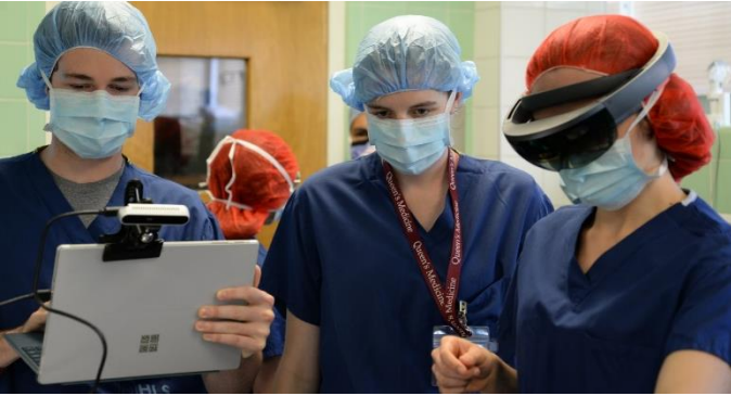
Fig. 3. Trainee (right) using the HoloLens to indicate the drill location and drill angle as a 3D point cloud of the scene is acquired using the Intel RealSense D415 Depth Camera (left).
