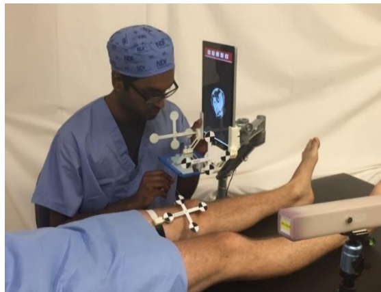
Figure 2: Participant using the system and adjustable table-mounted arm to plan a needle insertion path.
