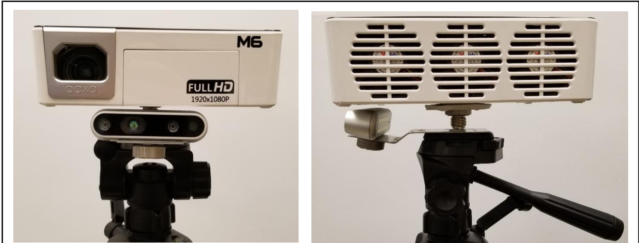
Figure 1. Front view [left] and side view [right] of the Pico M6 projector rigidly fixed to the Intel RealSense.
