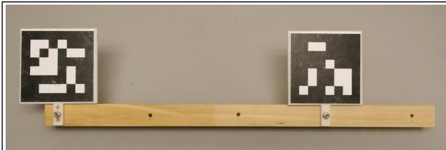
**Fig 9.** Measurement setup for assessing relative error.
