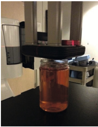
Fig. 1 Photo of a Fricke xylenol orange gel dosimeter positioned beneath a 6 \times 6 cm 2 field electron beam applicator
